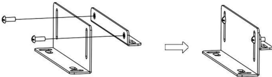
**Note:** You can adjust the bracket anywhere along the axis of the hole connecting the pieces allowing a flush fit with the wall or enclosure the unit is installed on.
