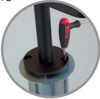
Align holes of the iPad holder to the post fixings. Insert and tighten 2 screws to secure. Rotate iPad holder through 90°, aligning remaining 2 holes to post fixings. Insert and tighten final screw to secure (in diametrically opposite hole from tightened screw in stage 8).
