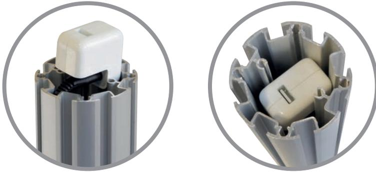
Position black mains cable into internal post channel and carefully slide USB Power Adapter down below the top of the post.
