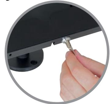
Unlock the iPad enclosure by inserting key into security lock and rotate "QUARTER TURN ONLY" clockwise or counter-clockwise through 90 degrees which releases the locking pin. Return key back to original position to remove.
